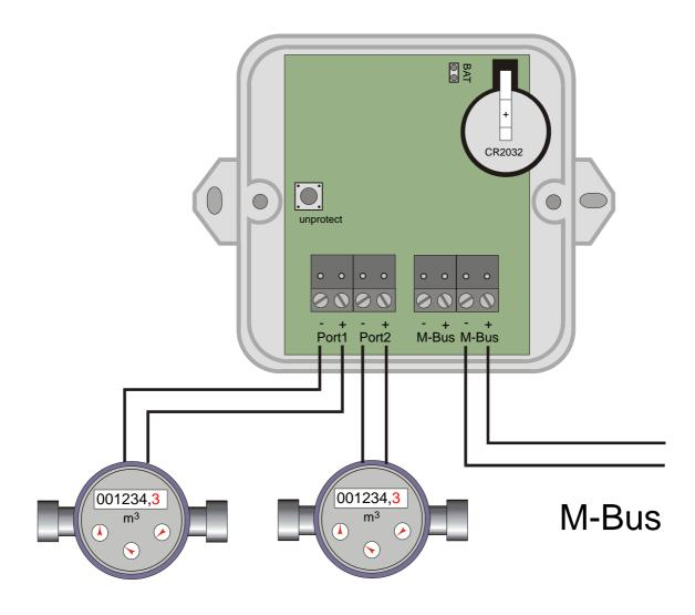
If not all ports of PadPulse M2 are used, you should not attach a cable to the respective unused port. The capacity of an open-circuited cable reduces the lifetime of the battery in stand-alone operation (no M-Bus available). The following graph represents the diagram of connections in the tariff mode with one counter and a tariff signal generator:
