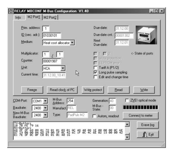
These sheet shows the current settings and values of the respectively pulse channel (port) of the PadPuls M2 (in this example: Port 1). The following input boxes and buttons are used to change the params of the pulse adapter:
