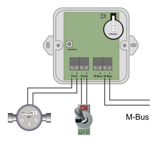
The specifications of the impulse and tariff signal generator can be taken from the technical data. The maximum pulse frequency to be counted is 14Hz.
