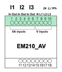
Measurement on three-phase systems without neutral (always self-power supply).
