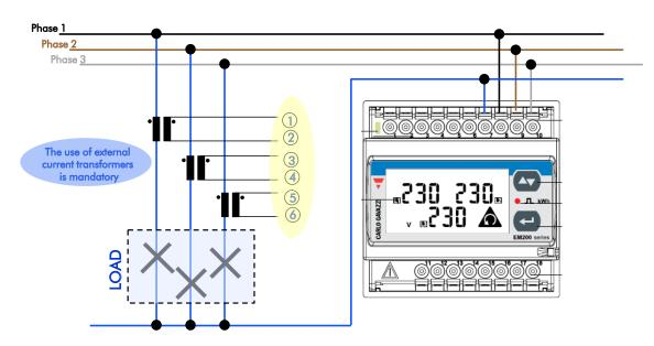
3-phase + N unbalance system (3 CT connection)
