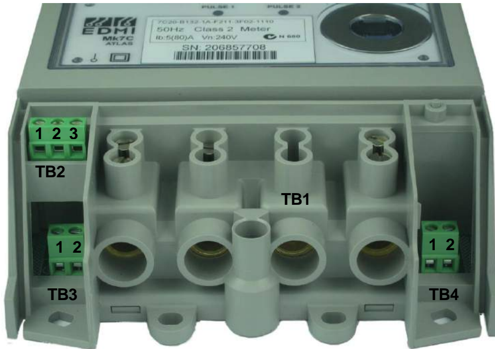
• Figure 6-8 Under the terminal cover of the meter
