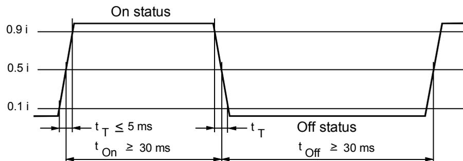
Figure 1. Pulse shape according to DIN 43 864
