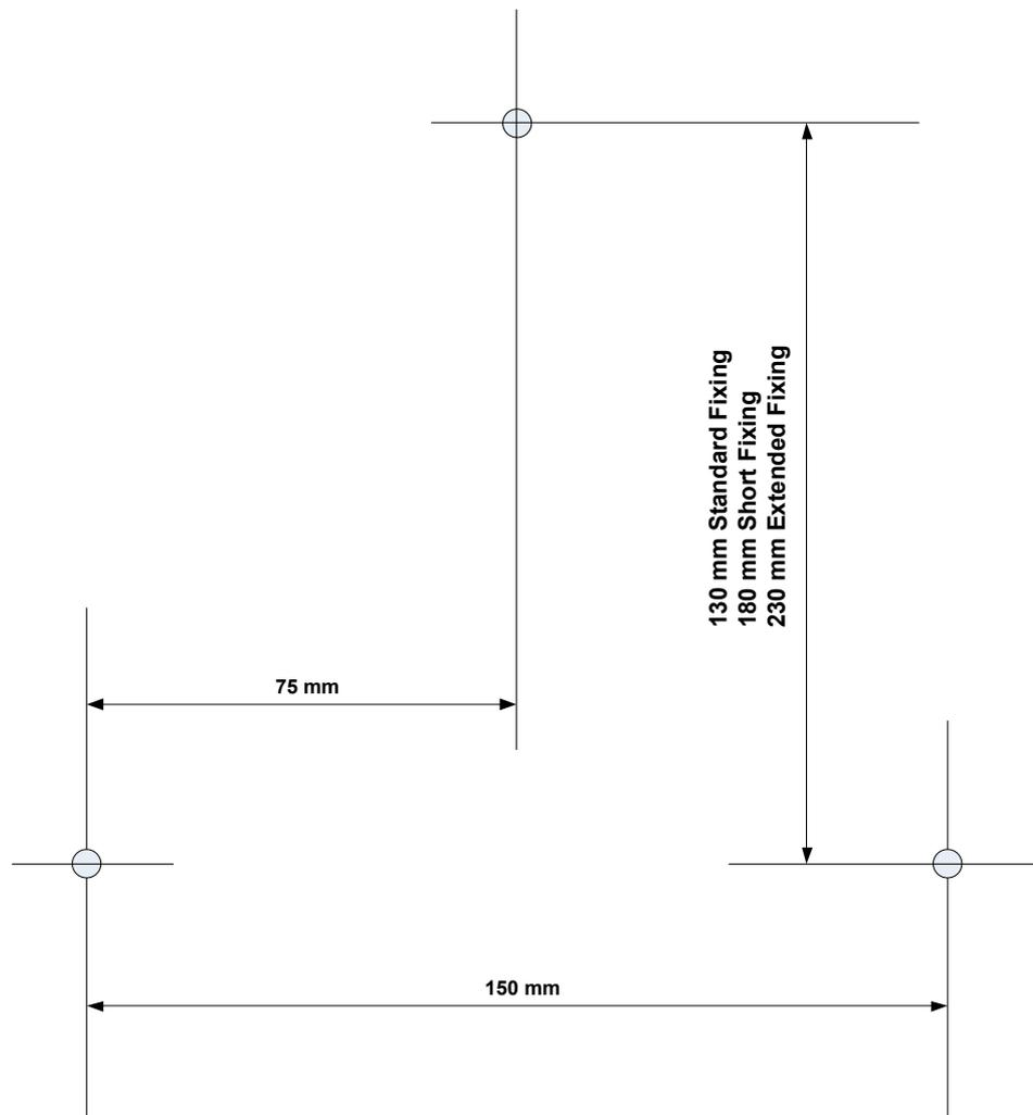
Figure 13. Drilling diagram for fixing screws
