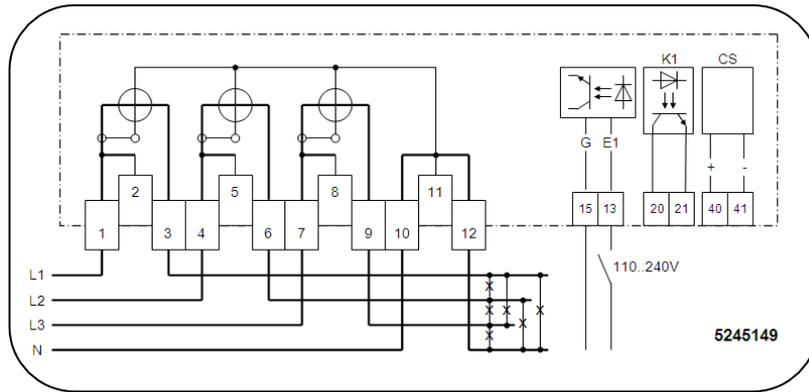
Figure 9. E230 3-phase 4-wire network, 1 pulse input, 2 pulse outputs and CS
