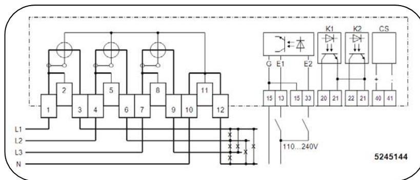
Figure 10. E230 3-phase 4-wire network, 2 pulse inputs, 2 pulse outputs and CS
