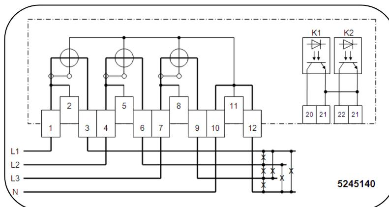
Figure 8. E230 3-phase 4-wire network, 2 pulse outputs
