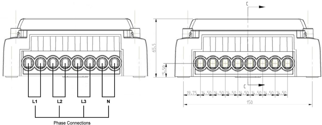
Figure 6. Terminal layout and phase connections
