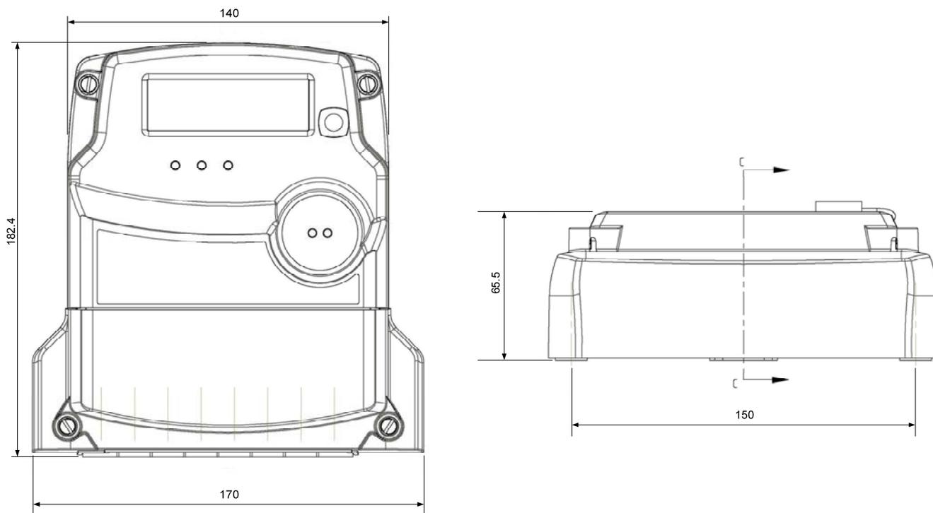
Figure 5. Meter with standard terminal cover and extended fixing bracket
