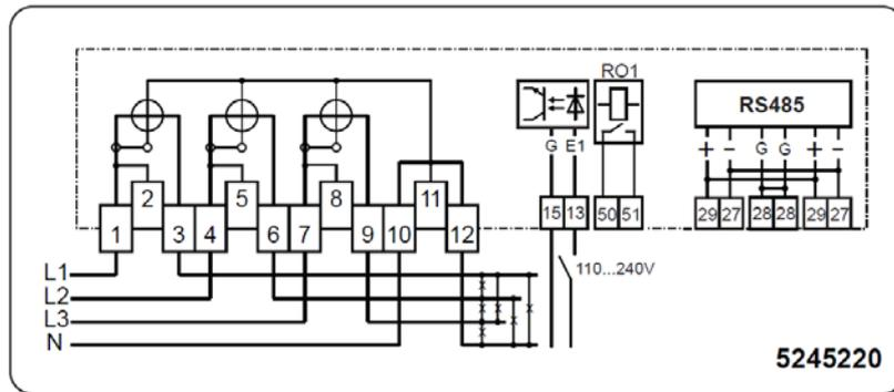
Figure 11. E230 3-phase 4-wire network, 1 pulse input, 1 relay output and RS485
