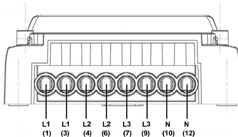
Figure 14. Phase connection diagram
