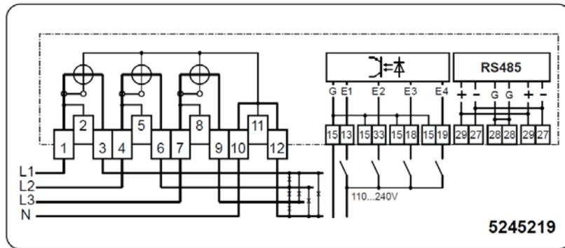
Figure 12. E230 3-phase 4-wire network, 4 pulse inputs and RS485
