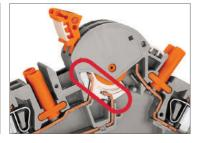
The measuring instrument is electrically disconnected from the transformer. In this position, if necessary, external voltage can be applied via sockets, or the 2nd CAGE CLAMP® connection for relay testing in transformer protection circuits.
