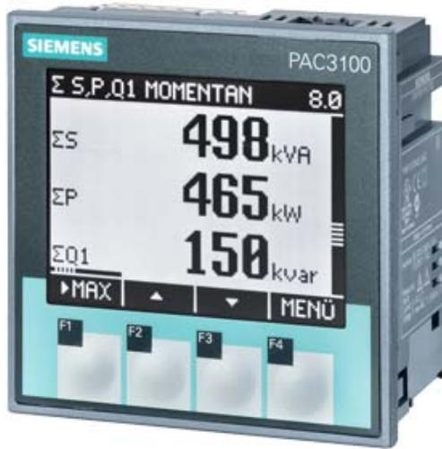
SENTRON PAC3100; LCD; 96X96MM POWER MONITORING DEVICE PANEL MOUNT TYPE FOR MEASUREMENT OF ELECTR. VALUES UC: 110-250VDC / 100-240VAC UE: MAX.480/277V; 45-65HZ IE: X/5A AC TERMINAL CONNECTION
