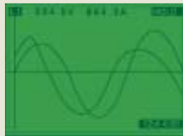
Scope function allows viewing of current and voltage waveforms.
